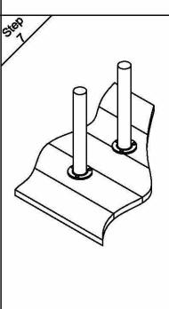
Place the longer of the tubes over the pipe flanges
