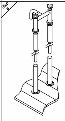
Place the tap/feed tube assembly over the floor tubes. The under floor pipework will determine the height of the fitting
